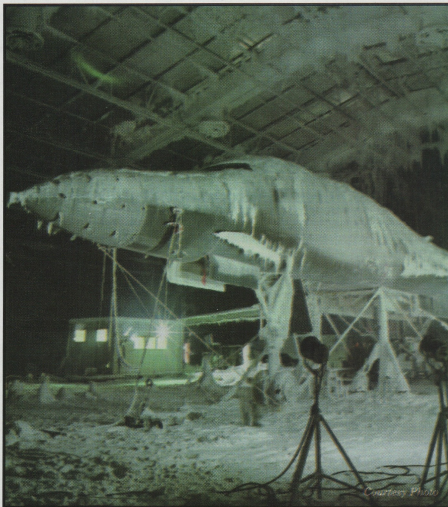
A B1-B Lancer undergoes testing at the McKinley Climatic Laboratory.
