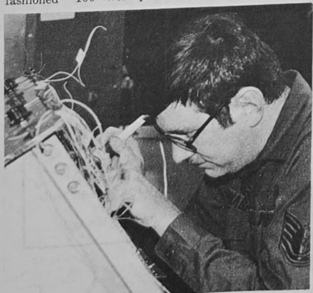
TSgt Doug McQuaid, NCOIC Weather Maintenance, repairs the receiver from the GMD-4 tracking set.
