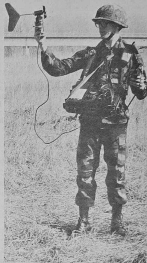
FIELD OBSERVATIONS — The essence of an accurate forecast is good observation. A1C. Daniel Gardner measures wind direction and speed with a TMQ-22 Tactical Observing Kit. (U.S. Army photo)
