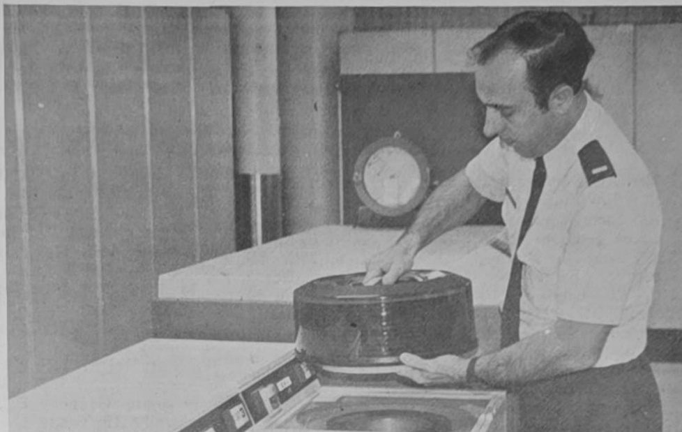
1ST LT. GARY WHITE installs a high speed disk on System 1. Lieutenant White is a computer operations officer who serves in a dual capacity as Air Force Global Weather Central's systems security officer and a systems duty officer. (U.S. Air Force photo)
