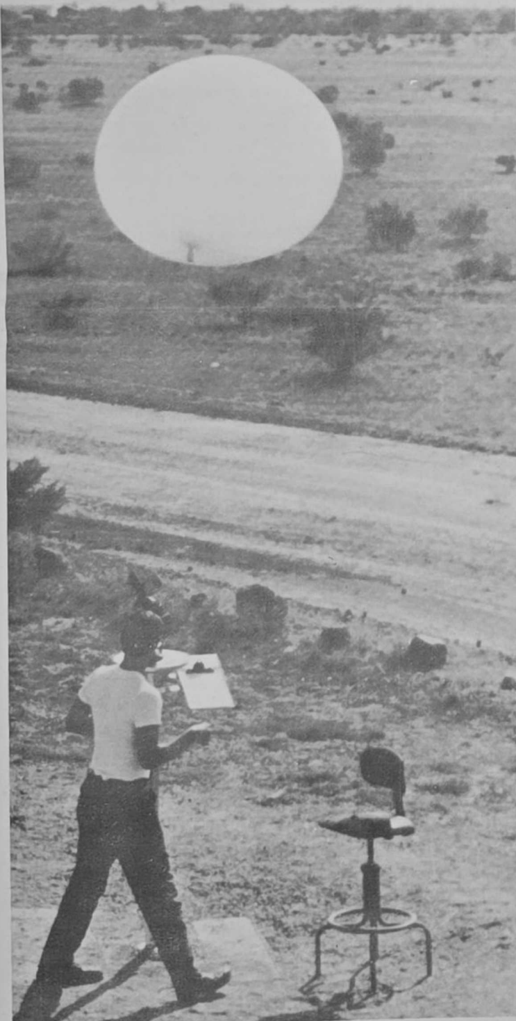
AMN. JOHN BURNS launches a 100-gram pibal from OL-A, Det. 15, 25th WS, Gila Bend AFAF, Ariz. Sand and sparse vegetation bear witness to the dryness and heat of this desert location. (U.S. Air Force Photo)
