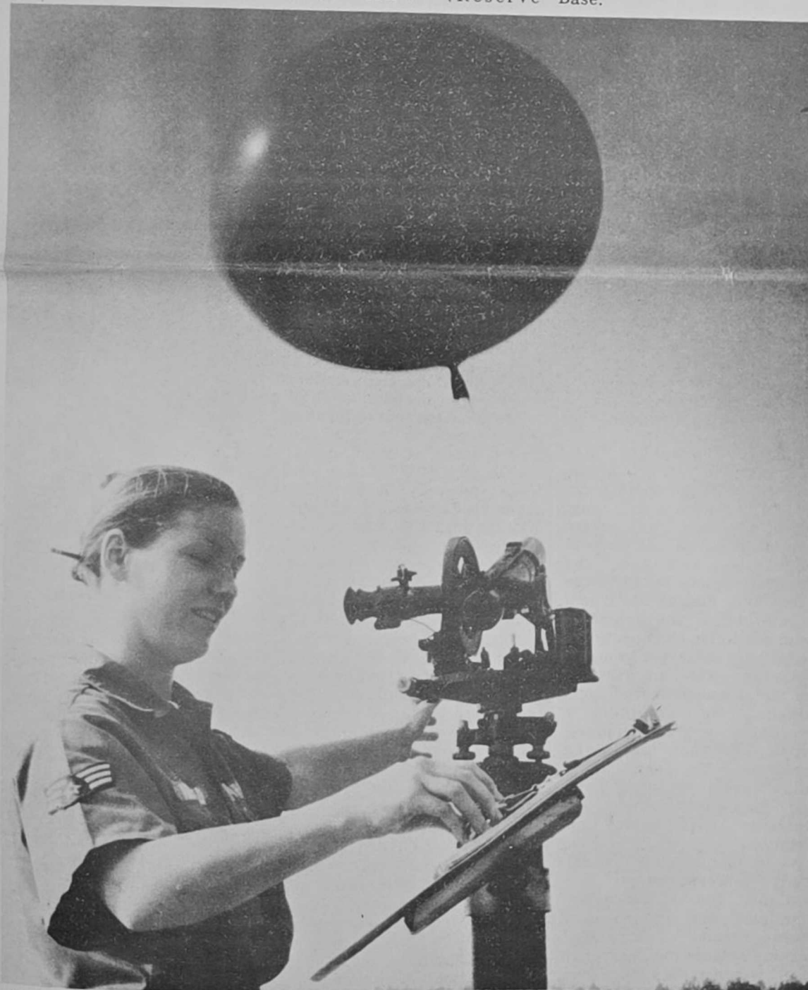
FIFTH WEATHER WING — Sgt. Victoria J. Archibald, Det. 1, 3rd Weather Squadron, Shaw AFB, S.C. prepares to take a Pibal sighting through the optical theodolite at the Poinsett
