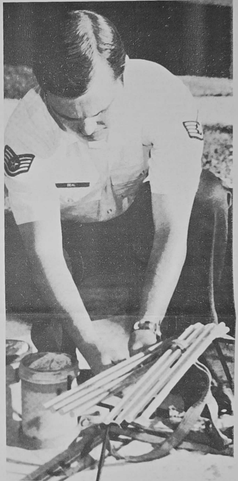
USING SPECIALLY designed fuel sticks and balance scales, SSgt. Daniel Deal of Det. 18, 25th Weather Squadron at Mountain Home AFB, Idaho, obtains data for determining the fire danger index at the Saylor Creek Bomb Range. (U.S. Air Force Photo)
