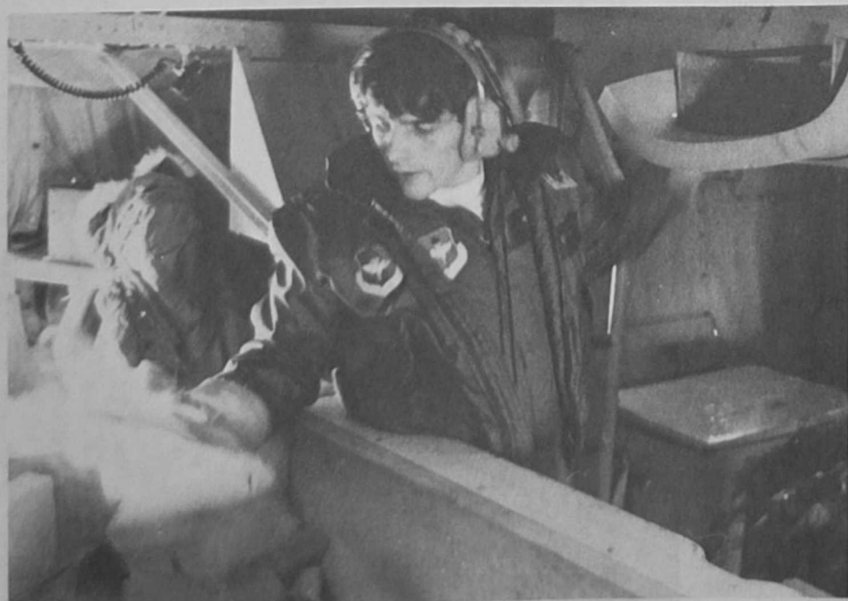
LOADING THE CHUTE is A1C Kelly Straight, a weather equipment repairman. The five-pound blocks of dry ice flow back to the rear of the aircraft to be crushed and used. (U.S. Air Force photo by Capt. James Perkins)
