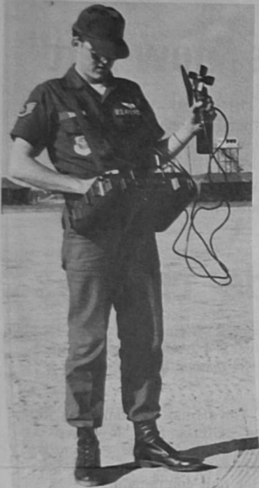
SSGT. RON SIMMEN takes and records an observation at Eglin AFB's Field Two using the new AN/TMQ-22 Tactical Observing Set. Sergeant Simmen is from Detachment 6, 3rd Weather Squadron, Homestead AFB, FL. (U.S. Air Force photo).
