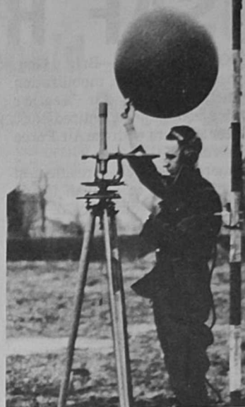
A MILITARY WEATHERMAN of the era between World War I and World War II uses a Theodolite and pilot balloon. The launch probed the atmosphere above the surface. Tracking was done using the three-legged Theodolite. (U.S. National Archives photo).
