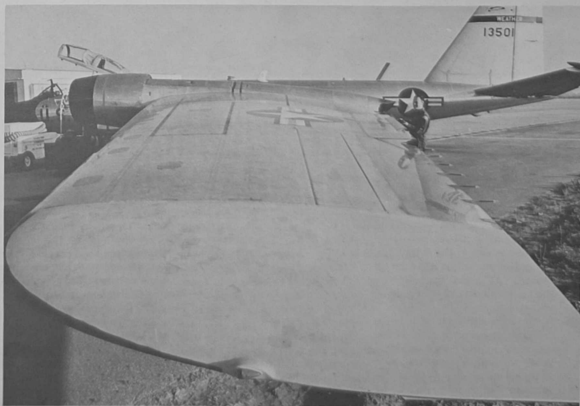
OUTSTRETCHED WING of an Air Weather Service WB-57F is checked by a pilot prior to flight. Each wing is doubled in length to permit flying at high altitudes. (U.S. Air Force Photo)
