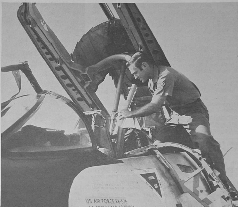
MR. FIXIT — Sgt. Donald E. Fix, 58th WRSq., installs a safety lock in the canopy of a WB-57F. Sergeant Fix is the Category 2 winner, MAC Aviation Maintenance Airman of the Year. (U.S. Air Force Photo)
