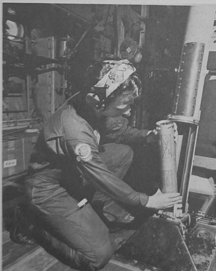
BELOW FLIGHT LEVEL, data is secured for winter-storm support in the same manner as AWS collects data on hurricanes, typhoons and other tropical storms, by dropsonde. Here a weather crewman prepares to drop one of the miniature weather stations, which automatically collect weather data as they fall by parachute and radio it back to the reconnaissance aircraft.
