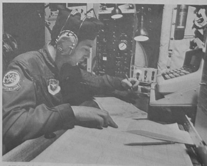
STORM DATA is evaluated by the airborne weather observer, TSgt. Robert Beaver, who also processes and encodes data from the falling dropsonde. This information, on pressure, humidity and temperature below flight level, is transmitted from the WC-130 by single-sideband radio to the ground weather network.
