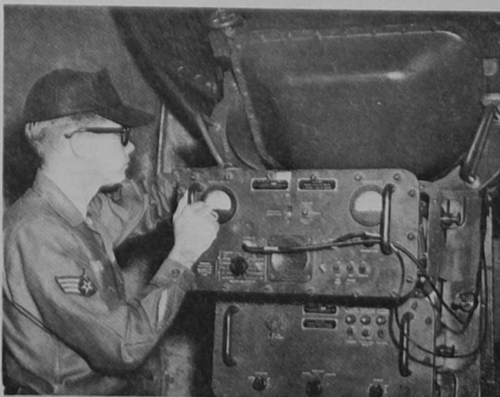
PULLING MINOR MAINTENANCE on a GMD-2 rawinsonde tracking set during a rawinsonde observation at Wheelus AB, Libya, is Sgt. Charles D. Everett, Detachment 13, 21st Weather Squadron. Det 13 will deactivate next month.
