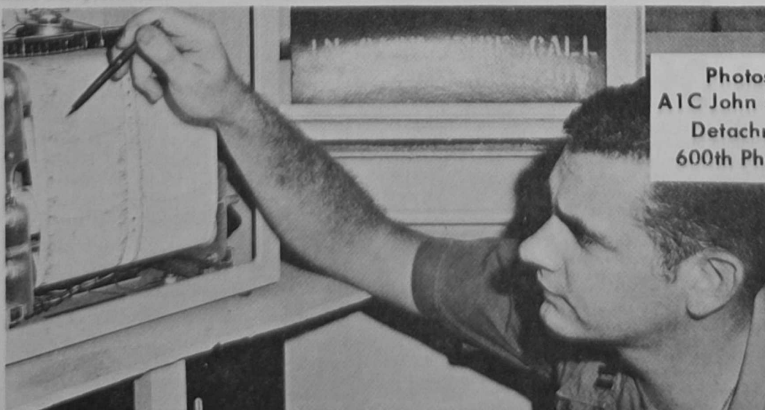
WIND-WATCHING, Capt. Senator C. Raygor studies the changes in wind direction near Bien Hoa from the wind direction recorder in the base
