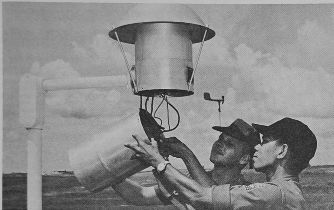
CHECKING THE HUMIDITY, TSgt. Billy F. McHenry (right), shows Republic of Vietnam Air Force (VNAF) SSgt. Nguyen Dinh Cuong readings on the temperature and humidity set
