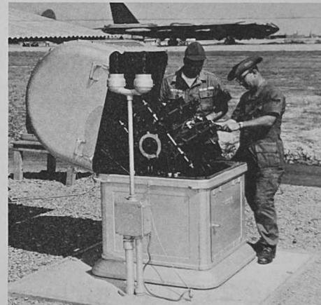
MAKING MINOR ADJUSTMENTS to the projector of the Rotating Beam Cellometer (cloud measurer) at U Tapao AB, Thailand, are Sergeants Raymond J. Metzger (left) and Robert W. Stalker, both members of Detachment 30, 10th Weather Squadron. Landing in the background is a war-painted B-52 Stratofortress.
