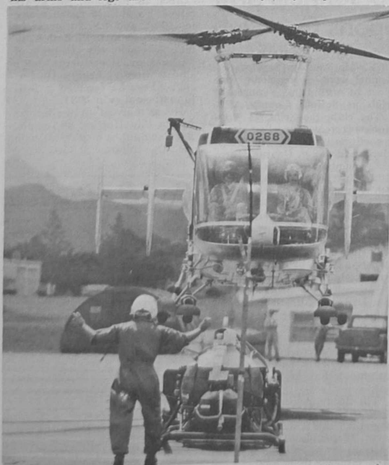
MOVING UP ON THE SPUTNIK is a delicate job. In seconds the Huskie—with its fire suppression kit slung underneath—will be speeding to the scene of an emergency landing. The Sputnik contains 688 gallons of foam—54 seconds of protection for the firefighters and crash victims.
