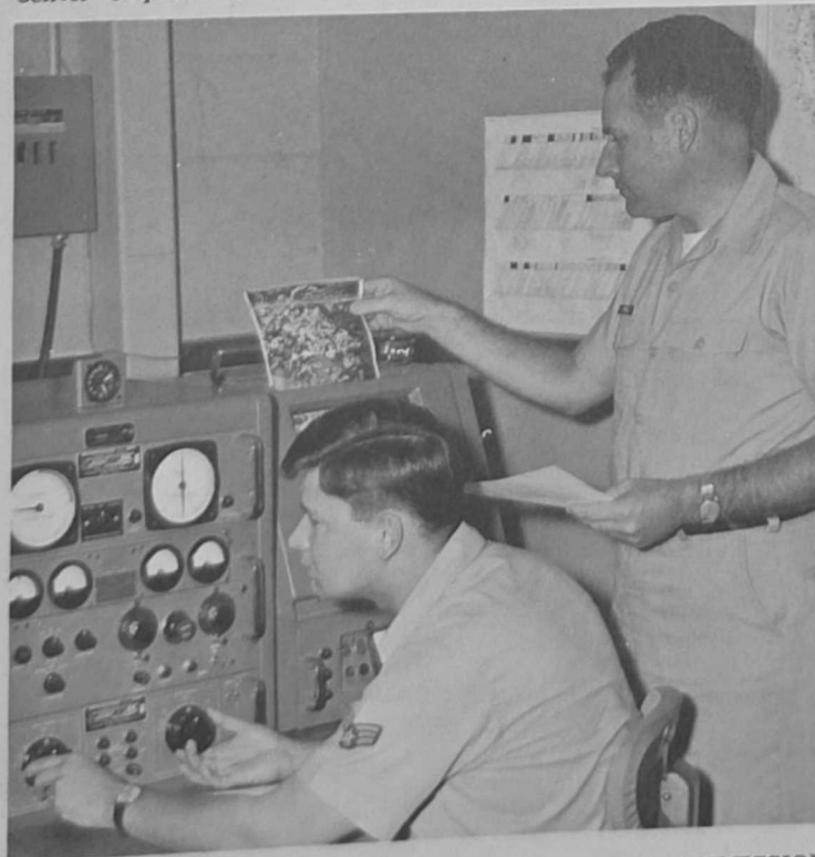
DET. 3 HAS AN AUTOMATIC PICTURE TRANSMISSION GROUND STATION which receives, records and displays cloud cover photographs taken and transmitted from an orbiting weather satellite. A1C Wesley M. Bennett (seated) operates the controls while TSgt. Edward N. Tidwell monitors reception. These weather pictures from space are valuable in the Pacific where vast stretches of ocean limit the density of surface observation stations.
