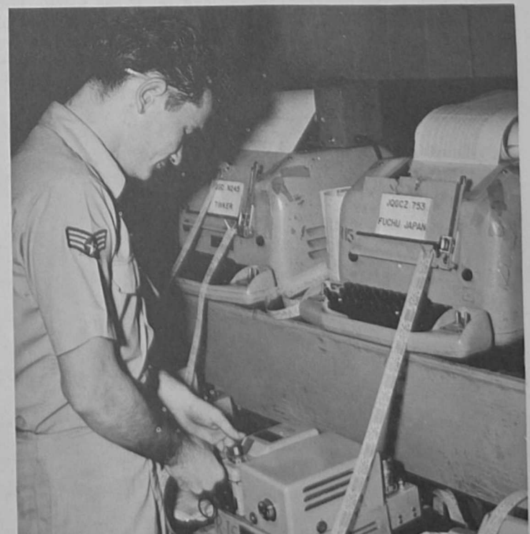
DET. 3 RECEIVES COOPERATION FROM AFCS which operates the unit's communications complex. AFCS operator A1C Terry L. Cunningham feeds weather information to a transmitting device which flashes the data—via teletype—to a 1st Weather Wing unit at Fuchu AS, Japan.
