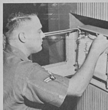
WEATHER EQUIPMENT REPAIRMAN A2c John Cullingford makes a periodic check on the wind direction and speed indicator located in the forecasting section of the Howard AFB Operations building.
