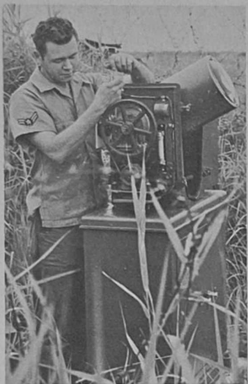
WEATHER EQUIPMENT REPAIRMAN , A2c Bruce A. Kibben, lends his skills to the AN/GMQ-2, Fixed Beam Ceilometer, at Detachment 10, 1st Weather wing, Kunsan, Korea. The barbed wire is to protect the instrument from being damaged by heavy Korean construction equipment.
