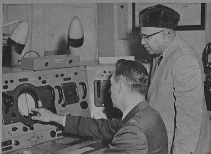
PAKISTAN WEATHERMAN, Mr. Muhammed Samiullah, deputy chief of the Pakistan Civil Weather Service, pauses during his tour of the Scott AFB, weather station to observe a CPS-9 storm detector radar unit, which accurately measures cloud heights and locates storms up to 300 miles away. Indicating its operation is Lt. Col. Fred J. Franz, operational requirements division, AWS Hq.
