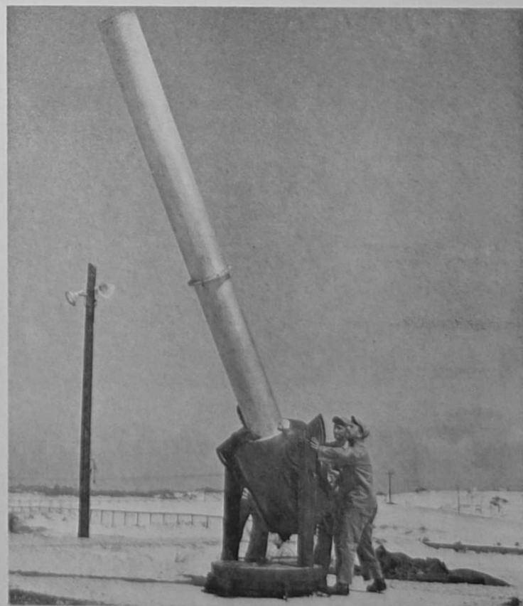
LAUNCHER containing the Arcas-Robin rocketsonde for obtaining high-altitude weather data is aimed skyward at Air Proving Ground center's Santa Rosa island launch site. The aimers are SSgt Robert L. Basius (left) and SSgt Charles L. Herron of APGC's high-altitude test probe branch.
