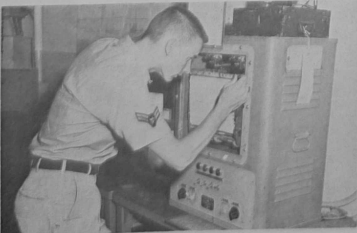
READING INFORMATION from the Ceilometer recorder is A/2c Danny Goins, Det. 11 observer. The ceilometer projects a beam that is used in measuring the bases of clouds.
