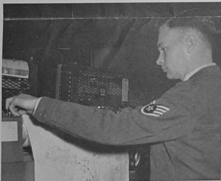
WEATHER OBSERVER SSgt Robert E. Curle prepares to transmit a Horizontal Weather Depiction chart (HWD) on the facsimile transmitter before sending it over the European weather facs circuit. The HWD shows weather conditions between 6,000 and 20,000 feet over the Atlantic.
