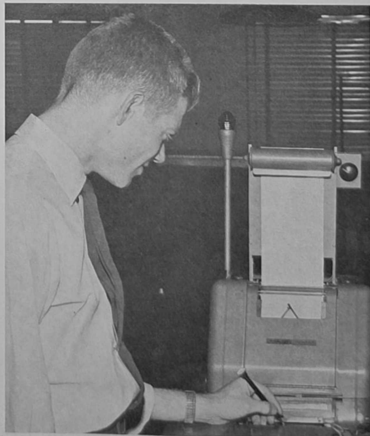
TRANSMITTING a message on the telautograph which automatically sends and receives weather data between Sheppard AFB and the US Weather Bureau at Kelly Field, is A/1c John H. Hirsch, an observer.
